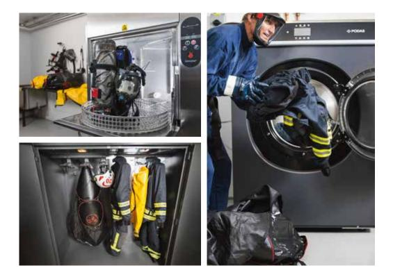
A smart solution for the thorough decontamination and cleaning of compressed air breathing apparatus is to machine wash.
