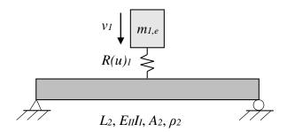
*Figure 5.6* The model used in the first ADINA analysis (ADINA model 1), with a point mass hitting a beam.
