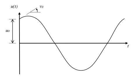
*Figure 3.11 Free vibration of an undamped SDOF system.*
