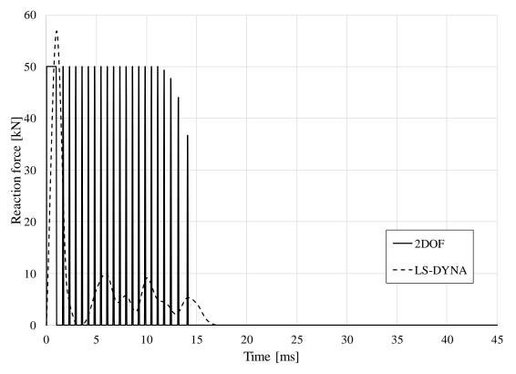
Figure 6.3 Reaction force of 2DOF and LS-DYNA model only.
