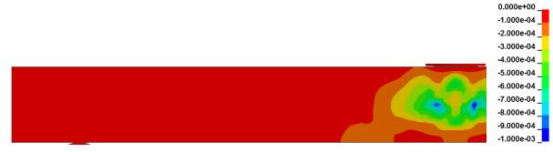
*Figure 6.25* 3<sup>rd</sup> principle strain (compression) 0.07 ms after impact.
