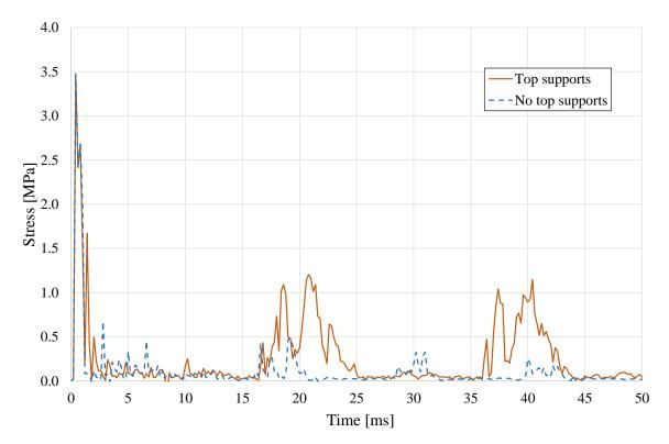
*Figure 7.12* Stress in the x-direction in the upper side of the beam as a function of time, shown for both support cases.
