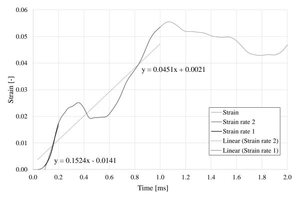
*Figure H.6* Strain as a function of time for an element where a bending crack was initiated.
