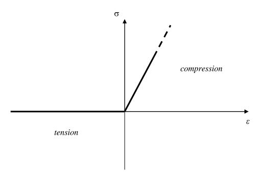
Figure 5.13 Behaviour of spring in the FE-models.
