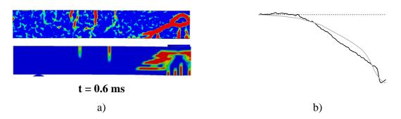
*Figure 6.37 Response after 0.6 ms: a) Crack pattern for RPC2 and LS-DYNA, respectively and b) Displacement shape for RPC2 (black) and LS-DYNA (grey).*
