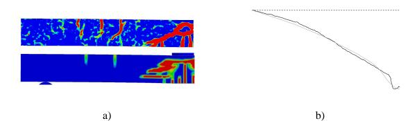
*Figure D.31 Response after 1.0 ms: a) Crack pattern for RPC2 and LS-DYNA, respectively and b) Displacement shape for RPC2 (black) and LS-DYNA (grey).*
