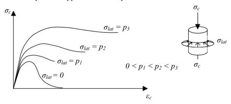
*Figure 2.10* The influence of lateral confinement on concrete in compression, from (Ekengren et al. 2005).
