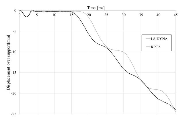
Figure 6.18 Beam displacement over the support over time, results from RPC2 and the LS-DYNA model.
