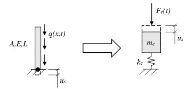
*Figure 4.8 A bar transformed into an equivalent SDOF system.*
