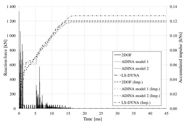
*Figure 6.2 Reaction force/Accumulated impulse (denoted as imp.) for the analytical models.*
