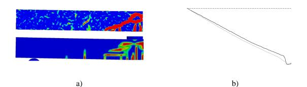
*Figure D.34 Response after 1.6 ms: a) Crack pattern for RPC2 and LS-DYNA, respectively and b) Displacement shape for RPC2 (black) and LS-DYNA (grey).*
