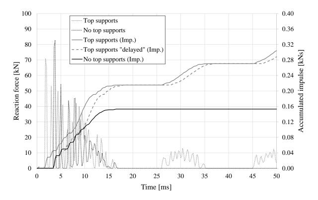
*Figure 7.9 Reaction force and accumulated impulse in the beam - bottom support interface for both the model with top supports and without.*
