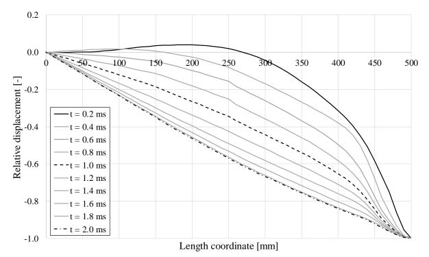
*Figure 6.32* Displacement shape of the beam in the LS-DYNA model with no supports during the first 2 ms.
