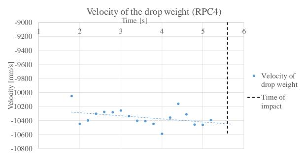
Figure D.26 Derivation of a value for the velocity at impact in the experiment.
