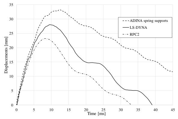
Figure 7.18 Displacement of midpoint over time.
