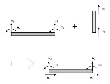
*Figure 5.9 Degrees of freedom for a beam element in ADINA.*
