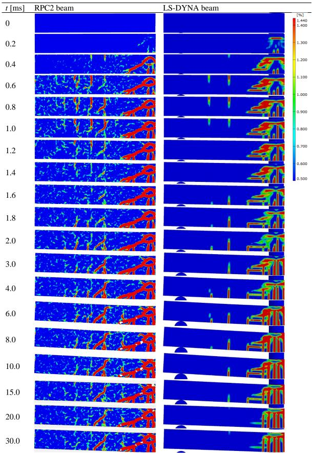
Table 6.51st principal strain showing crack patterns of RPC2 and LS-DYNA model at<br/>various time steps. Note that the time steps do not increase linearly in the table.
