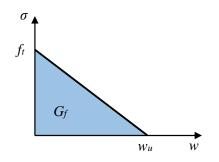
*Figure 5.20 A linear damage curve for the CDPM2 material model.* The crack width is calculated using equation (5.20).
