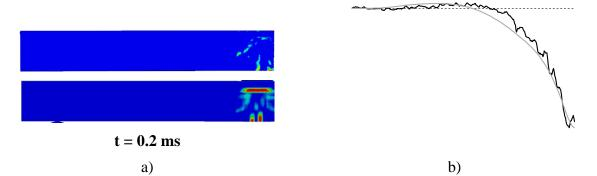
Figure 6.35 Response after 0.2 ms: a) Crack pattern for RPC2 and LS-DYNA, respectively and b) Displacement shape for RPC2 (black) and LS-DYNA (grey).
