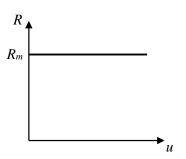
*Figure 2.4 The internal resisting force and displacement relation for an ideal plastic material.*
