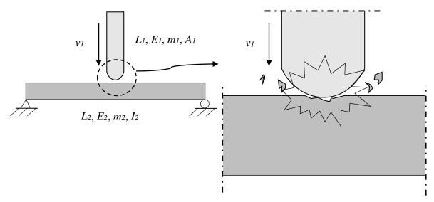
*Figure 4.12 The beam-drop weight system and the equivalent transformed mass-spring system.*
