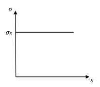
Figure 2.3 Stress-strain relation for an ideal plastic material.
