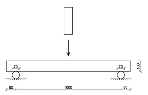
Figure 5.1 Test set up showing the beam geometry and boundary conditions.
