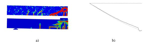
Figure D.35 Response after 1.8 ms: a) Crack pattern for RPC2 and LS-DYNA, respectively and b) Displacement shape for RPC2 (black) and LS-DYNA (grey).
