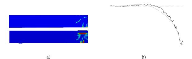
Figure D.27 Response after 0.2 ms: a) Crack pattern for RPC2 and LS-DYNA, respectively and b) Displacement shape for RPC2 (black) and LS-DYNA (grey).
