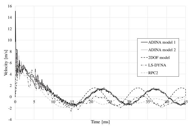
*Figure 6.1 Velocity over time for midpoint of the beam.*
