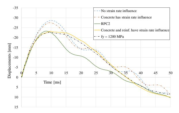
*Figure 7.15 Displacement of midpoint as a function of time including response of the beam with reinforcement with increased yield strength.*
