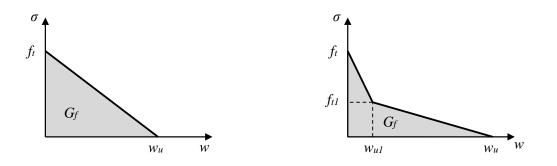
a) Linear fracture energy damage model b) Bilinear fracture energy damage model Figure 7.1 Two fracture energy damage models used in CDPM2.
