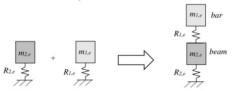
Figure 4.10 Two SDOF system becomes one 2DOF system.
