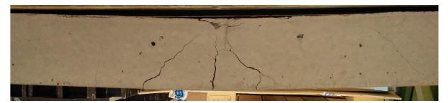
*Figure 6.24 Crack pattern displaying a horizontal crushing crack, shear cracks and bending cracks. Photo by Erla Sara Svavarsdóttir.*
