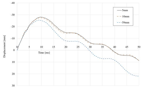
*Figure H.5* Displacement of the middle of the beam as a function of time for three different mesh sizes.
