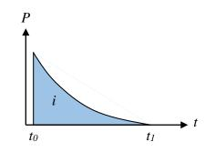
*Figure 3.2 Impulse intensity.*
