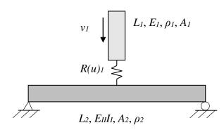
*Figure 5.7 The model used in the second ADINA analysis (ADINA model 2), with a rod hitting a beam.*
