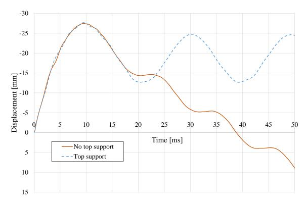
*Figure 7.6 Displacement of midpoint as a function of time for two different support conditions.*
