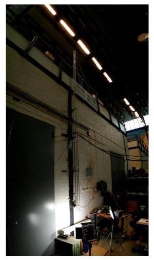
*Figure 5.3 Test set up showing the drop weight device. Photo by Erla Sara Svavarsdóttir.*
