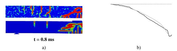
*Figure 6.38 Response after 0.8 ms: a) Crack pattern for RPC2 and LS-DYNA, respectively and b) Displacement shape for RPC2 (black) and LS-DYNA (grey).*
