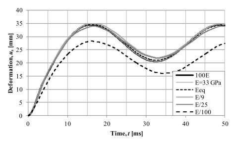
Figure 5.12 Study of the influence of different E for the response of a beam subjected to a point load (Andersson & Karlsson 2012).
