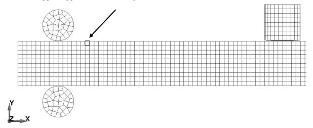
Figure 7.11 Element chosen for stress investigation.
