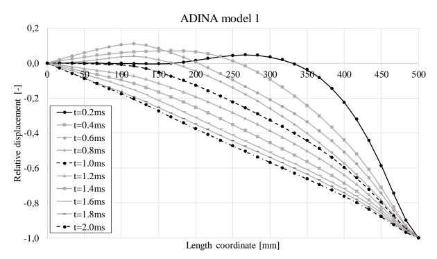
*Figure D.4 Displacement over length of ADINA model 1.*
