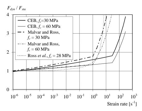
*Figure 3.27* Different studies of the dynamic implification factor-strain rate relations for concrete in tension. (Johansson 2000)
