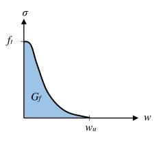
Figure 2.12 Internal work for elastoplastic materials, where  $w_u$  is the maximum crack width when the stress reaches zero.
