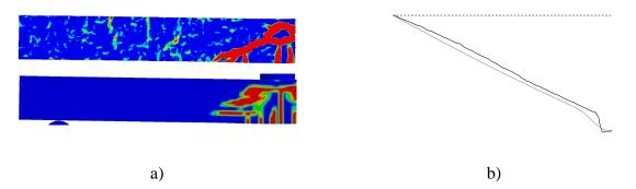
Figure D.33 Response after 1.4 ms: a) Crack pattern for RPC2 and LS-DYNA, respectively and b) Displacement shape for RPC2 (black) and LS-DYNA (grey).
