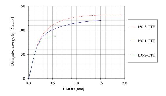
*Figure C.1* Accumulated fracture energy measured in three different test specimens.
