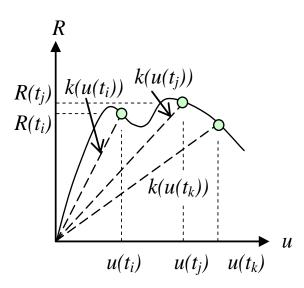
*Figure 3.25* Secant stiffness k at time t for a system with an arbitrary response (Johansson & Laine 2012).
