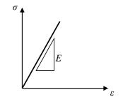
*Figure 2.1 Stress-strain relation for a linear elastic material.*
