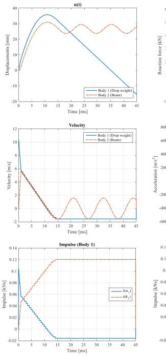
Figure D.1 Results from 2DOF model.
