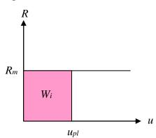
*Figure 3.6 Internal work for ideal plastic materials.*
