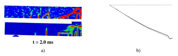
Figure 6.39 Response after 2.0 ms: a) Crack pattern for RPC2 and LS-DYNA, respectively and b) Displacement shape for RPC2 (black) and LS-DYNA (grey).
