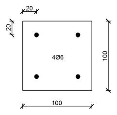
Figure 5.5 Cross section of the concrete beam.
