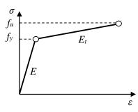
Figure 5.21 The bilinear elastoplastic behaviour of material model 003 – PLASTIC \_ KINEMATIC.
