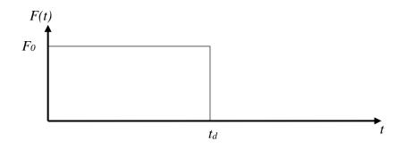
*Figure 3.15 Rectangular pulse input.*
