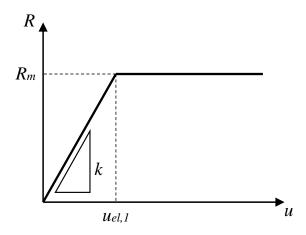
*Figure 2.5 The internal resisting force and displacement relation for an elastoplastic material.*
