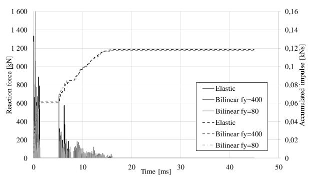
*Figure D.11 Comparison elastic/bilinear material response of the drop weight.*
