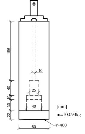
Figure 5.4 Cross section of the drop weight.
