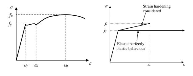
a) Stress-strain diagram. b) Idealised stress-strain behaviour.
