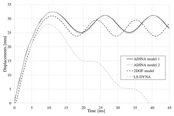
*Figure 6.8 Displacement of the midpoint from the different analytical models.*
