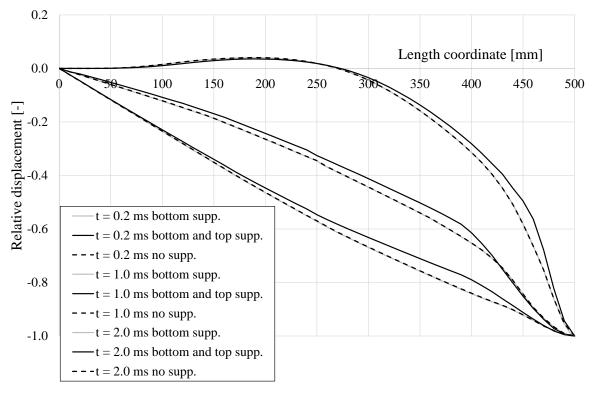
Figure 7.10 Displacement shape u(x) of a LS-DYNA modelled beam with three types of support conditions for three different time steps.
