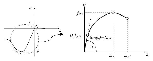
*Figure 2.8* Stress-strain relation of concrete in compression for structural analysis.
