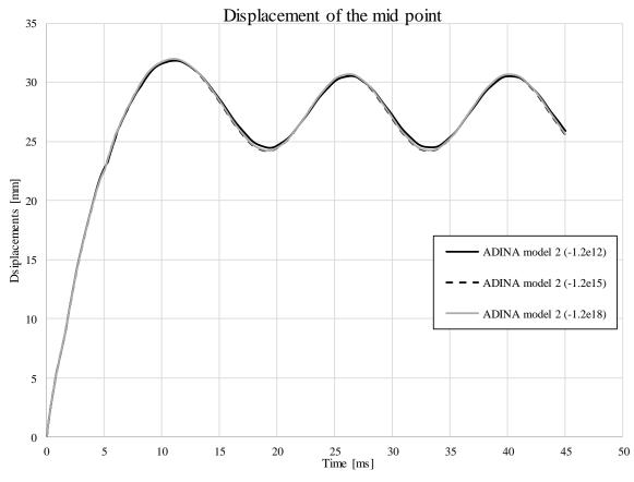
*Figure H.2 Response of midpoint using different spring stiffness for ADINA model 2.*
