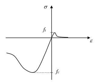
Figure 2.6 Stress-strain relationship for concrete.
