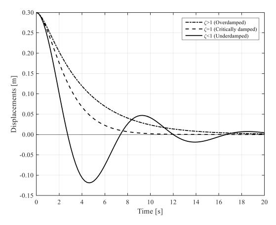
Figure 3.13 Vibration of a damped SDOF system.
