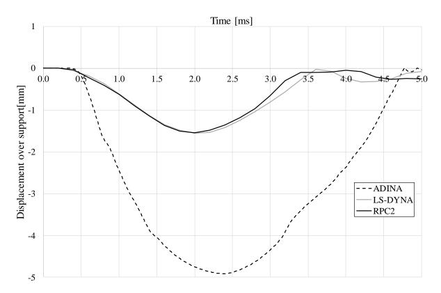
*Figure 6.21* Beam displacement over support during the first 4ms.
