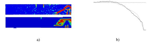
Figure D.28 Response after 0.4 ms: a) Crack pattern for RPC2 and LS-DYNA, respectively and b) Displacement shape for RPC2 (black) and LS-DYNA (grey).
