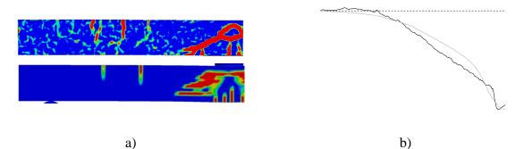
Figure D.29 Response after 0.6 ms: a) Crack pattern for RPC2 and LS-DYNA, respectively and b) Displacement shape for RPC2 (black) and LS-DYNA (grey).
