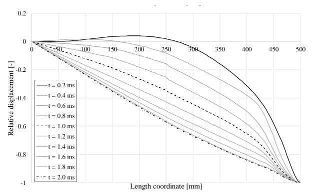
Figure 6.29 Displacement shape of the beam in the LS-DYNA model during the first 2 ms.
