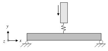
Figure 5.10 Boundary conditions for the FE-models in ADINA.
