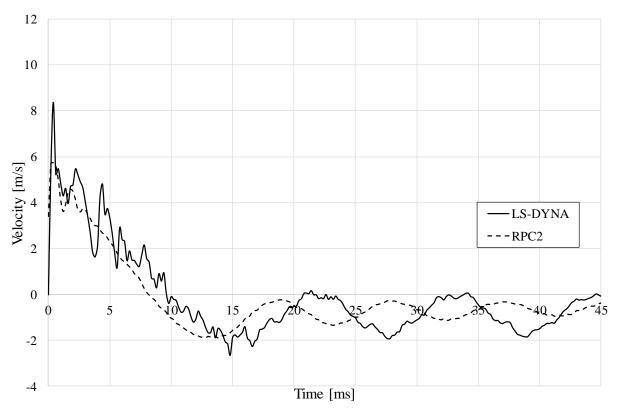
Figure 6.13 Velocity over time of the midpoint for the LS-DYNA model and RPC2.
