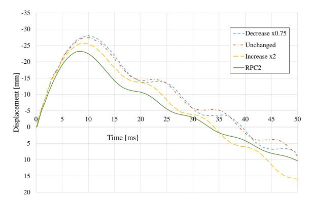
*Figure 7.4 Displacement as a function of time for three different magnitudes of fracture energy.*
