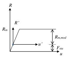
Figure 4.11 Influence of static loads on the dynamic response. Based on (Johansson 2014).*R<sub>m,mod</sub>* is then calculated as:
