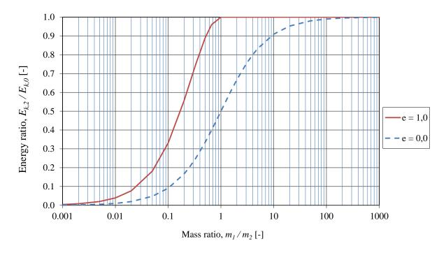
Figure 3.20 Energy ratio as a function of mass ratio for a purely elastic case (e=1) and a purely plastic case (e=0).
