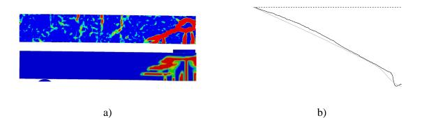
*Figure D.32 Response after 1.2 ms: a) Crack pattern for RPC2 and LS-DYNA, respectively and b) Displacement shape for RPC2 (black) and LS-DYNA (grey).*
