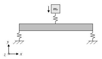
Figure 7.16 ADINA model with spring supports.
