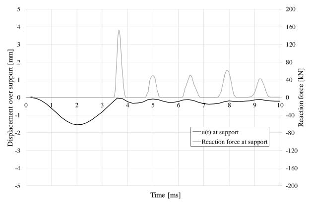
*Figure 6.31 Displacement over support/Reaction force of support during the first 10 ms from the LS-DYNA results.*
