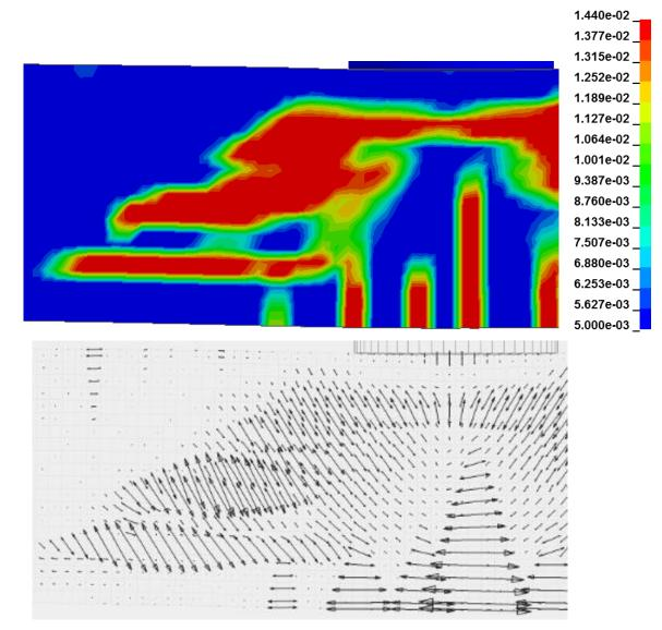
*Figure 6.23* 1<sup>st</sup> principle strain 0.8 ms after impact along with a vector plot showing the direction of the strain for the middle area of the beam.
