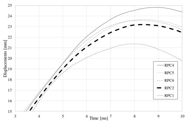
*Figure 6.7 Maximum displacement for the beams in the experiment, with RPC2 highlighted.*
