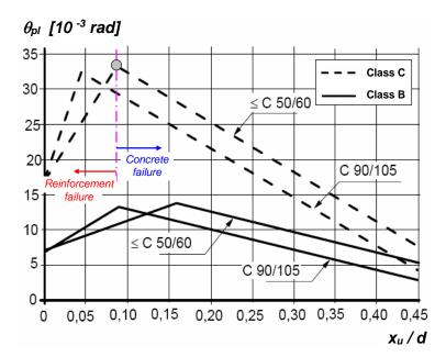
Figure 2.15 Design values for plastic rotation for various concrete and steel types, based on (CEN 2004). The limit between reinforcement failure and concrete failure in the case of concrete class  $\leq$  C50/60 and reinforcement class C is shown.
