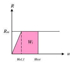
*Figure 3.7 Internal work for elastoplastic materials.*
