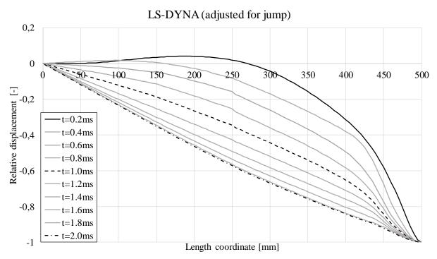
Figure D.14 Displacement over length for LS-DYNA model, adjusted for jump at supports-
