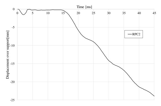
*Figure 6.15 Beam displacement by the support over time, where negative displacement represents the beam going in positive y-direction (vertical direction).*
