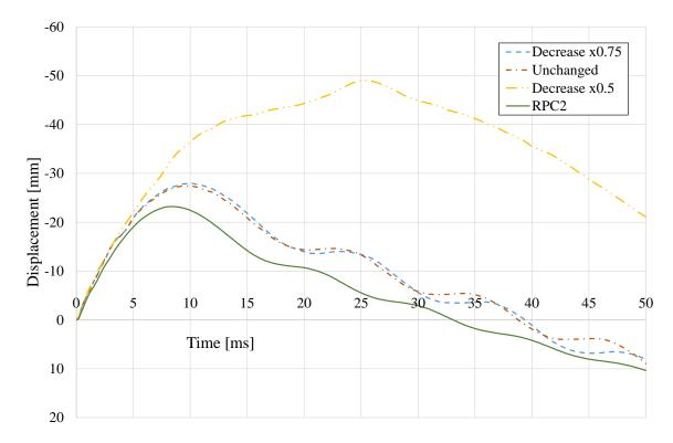
*Figure H.7* The midpoint displacement for three values of fracture energy along with the RPC2 test result.
