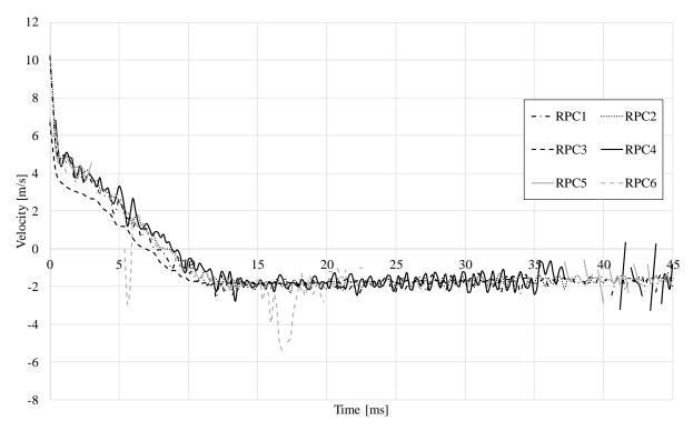
Figure D.24 Drop weight velocity of the beams in the experiment.
