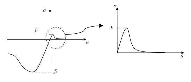
Figure 2.11 Stress strain relationship for concrete in tension
