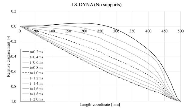
Figure D.15 Displacement over length for LS-DYNA model with no supports,
