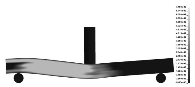
*Figure H.8* Beam shape from an LS-DYNA model where the fracture energy input has been reduced by x0.5.
