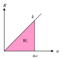
Figure 3.5 Internal work for linear elastic materials.
