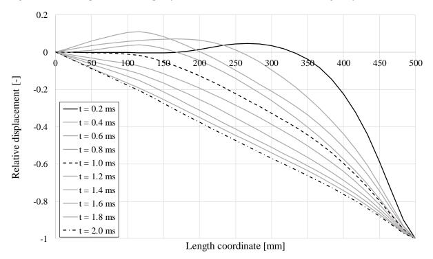
*Figure 6.28 Displacement shape of the beam in ADINA model 2 during the first 2 ms.*
