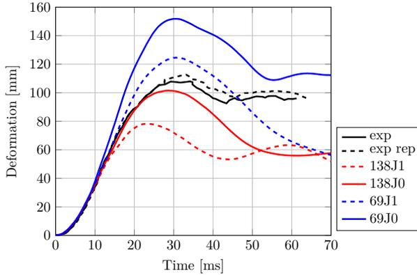
Figure 11: Deformation history for Blind simulation blast test for different fracture energies, 138 and 69  $\text{Nm/m}^2$ , and strain rate dependent strength turned on, 1, and off, 0.
