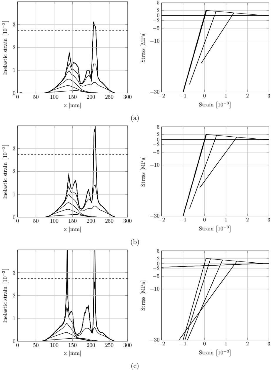
Figure 9: Mesh size sensitivity showing the distribution of inelastic strains for the damage-plasticity model through the wall at each time step  $\Delta t$  (left) and stress-strain response for the element with the highest inelastic strain (right), (a) coarse mesh  $N = 50$ , (b) original mesh  $N = 100$  and (c) fine mesh  $N = 200$ .
