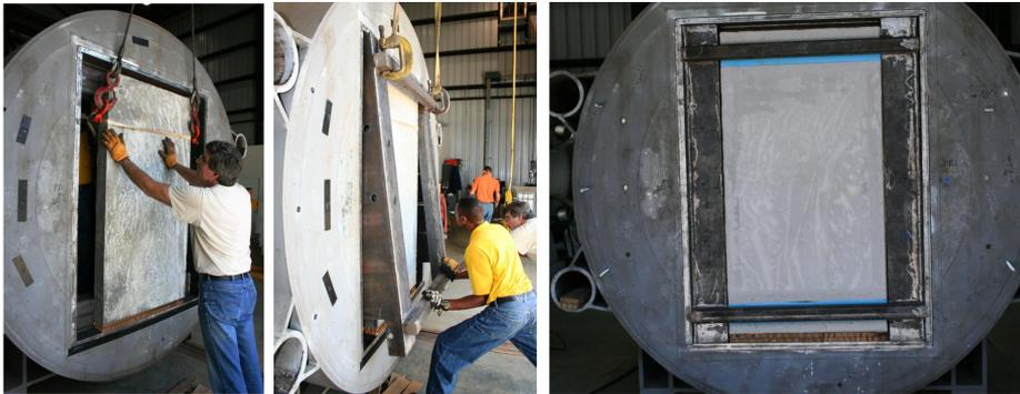
Figure 4: Mounting of Blind simulation slab with steel frame taken from competition input; also presented in [5]
