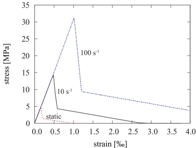
Figure 1: Softening branch for CDPM2 with dynamically increased tensile strength for different strain-rates taken from [2]
