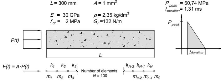
Figure 5: Geometry, boundary conditions and load.
