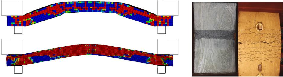
Figure 13: Failure mode before and after mesh refinement and crack pattern seen from the top (left) and the back side (right) of the slab; taken from [5].
