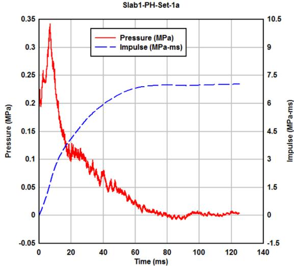
Figure 5: Measured pressure for blast load in Blind simulation blast test taken from competition input; also presented in [6] and [5]
