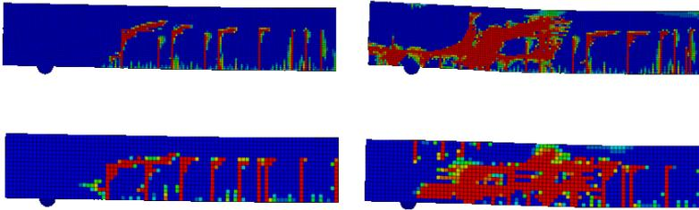
Figure 14: Shear crack near support for refined mesh (above) and for coarse mesh (below) for the FOI beam early (left) and late (right) in the analyses.
