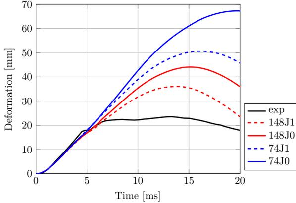
Figure 9: Maximum deformation vs time history for the analyses of the FOI beam for different fracture energies, 148 and 74  $\text{Nm/m}^2$ , and strain rate dependent strength turned on, 1, and off, 0.
