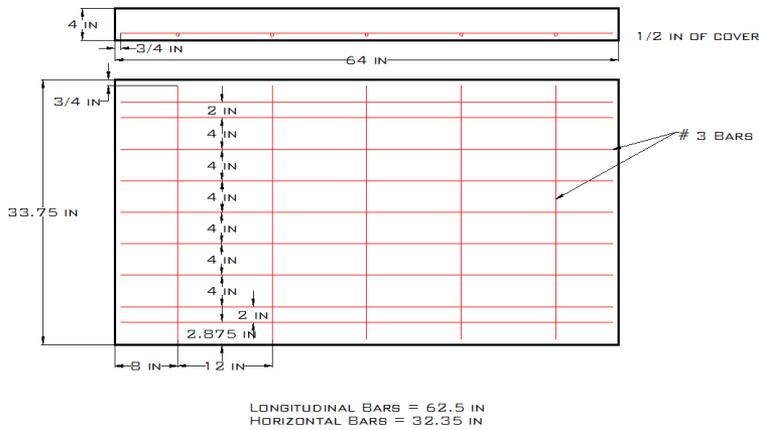
Figure 3: Reinforcement arrangement and geometry of Blind simulation slab taken from competition input; also presented in [6] and [5]
