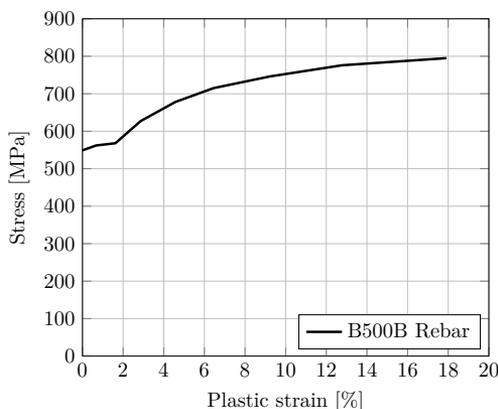
Figure 6: Stress-strain response of reinforcement for FOI beam adapted from [4]
