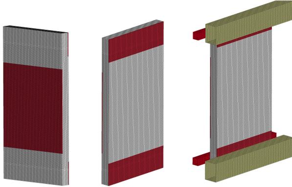
Figure 8: Elastic elements in the numerical model of the Blind simulation slab. Top side (left), bottom side with and without support structure (middle and right)
