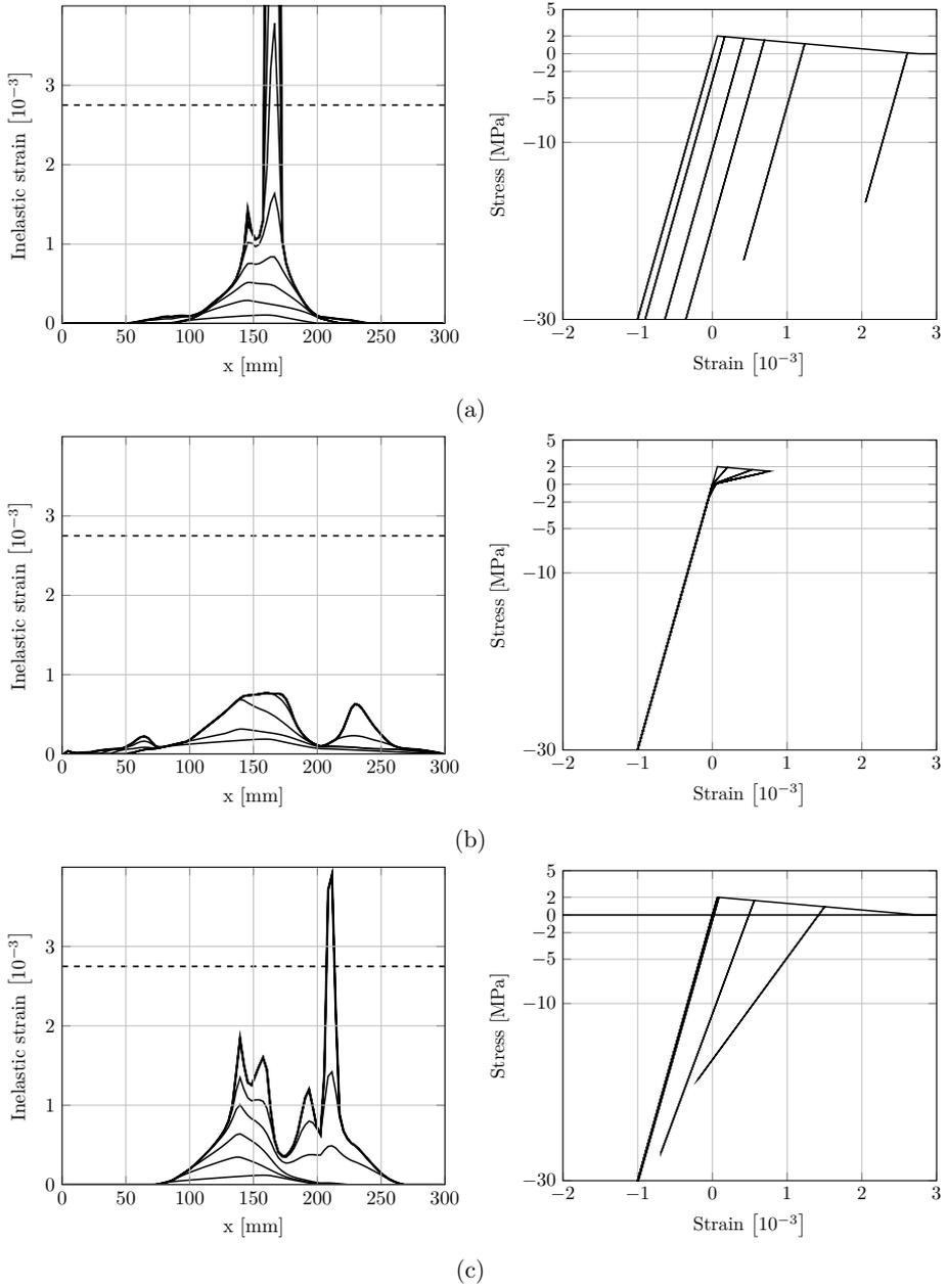
Figure 7: Response based on the finite element analysis showing the distribution of inelastic strains through the wall at each time step  $\Delta t$  (left) and stress-strain response for the element with highest inelastic strain (right), (a) for the plasticity model, (b) for the damage model and (c) for the damage-plasticity model.
