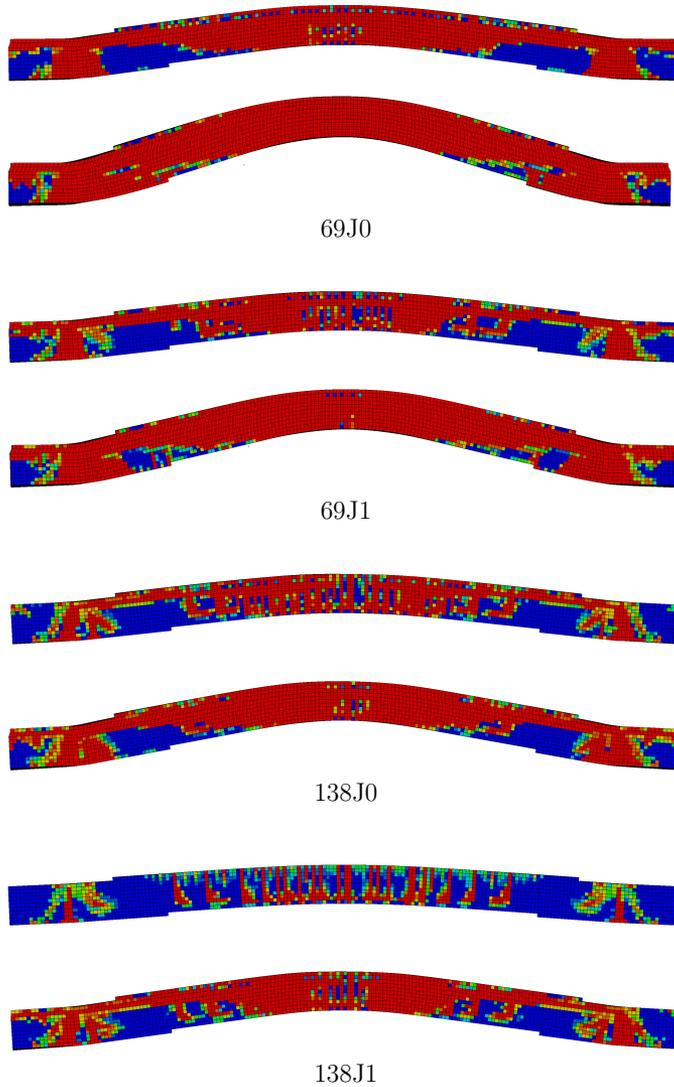
Figure 12: Contour plot of damage of the Blind simulation blast test slab for different fracture energies, 138 and 69  $\text{Nm/m}^2$ , and strain rate dependent strength turned on, 1, and off, 0. Top contour plots at the time of half maximum deformation and bottom plots at maximum deformation. Red colour represent full damage and blue represent no damage.
