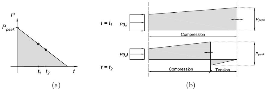
Figure 1: Illustration of (a) the applied pressure wave towards the left edge of the wall and (b) the stress distribution through the thickness of the wall when the pressure wave reaches the unloaded right edge of the wall (above) and at crack initiation (below).
