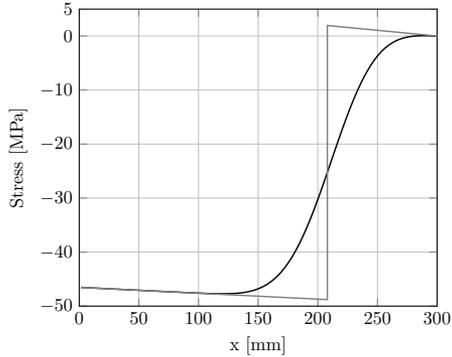
Figure 6: Stress distribution at the time of crack initiation for analytical solution. Stress distribution in numerical analysis (black) and analytical solution with jump condition (gray)
