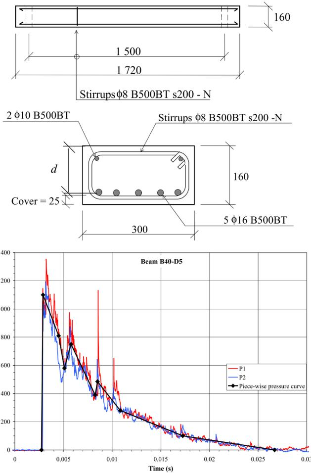
Figure 2: Geometry and reinforcement layout (above) and measured pressure over the beam and simplified load used in the analyses (below); both pictures taken from [4]
