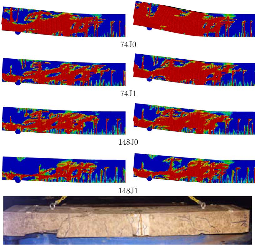
Figure 10: Contour plot of damage and the crack pattern of the tested beam (taken from [4]) for the FOI beam for the different fracture energies, 148 and 74  $\text{Nm/m}^2$ , and strain rate dependent strength turned on, 1, and off, 0. Left contour plots at the time of half maximum deformation and right plots at maximum deformation. Red colour represent full damage and blue represent no damage.
