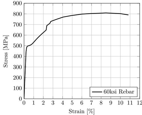
Figure 7: Stress-strain response of reinforcement adapted from competition input and [6]
