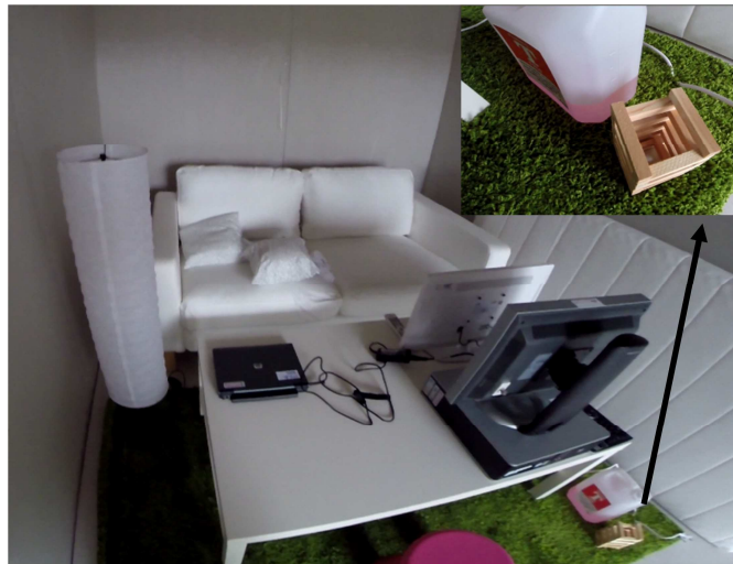
Figure 4. Picture of the container interior and the standardized ignition set-up (small picture)
