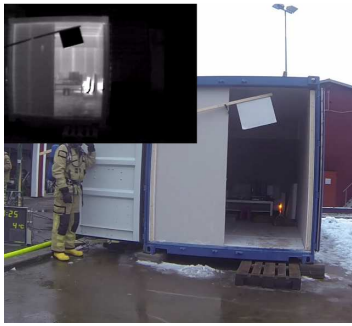
1. Fog spear with water. Varying winds, partly away from the container opening
