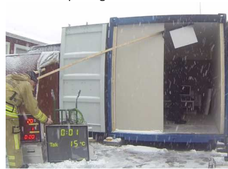
4. Cutting extinguishing with water and additive X-fog. Winds directed towards container opening
