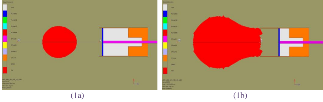
Fig. 17 TNT gas bubble in sand simulation group 9 with stiffness 0.1 MN/m and piston mass 5.2 kg. Material location at 18 ms (1a) and material localisation at 120 ms (1b). The scaled charge distance is 0.87 m/kg 1/3 and piston plate area is increased 300% in group 9.
